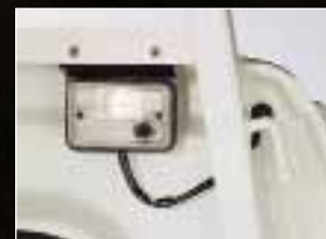
Cargo Deck Work Lamp
